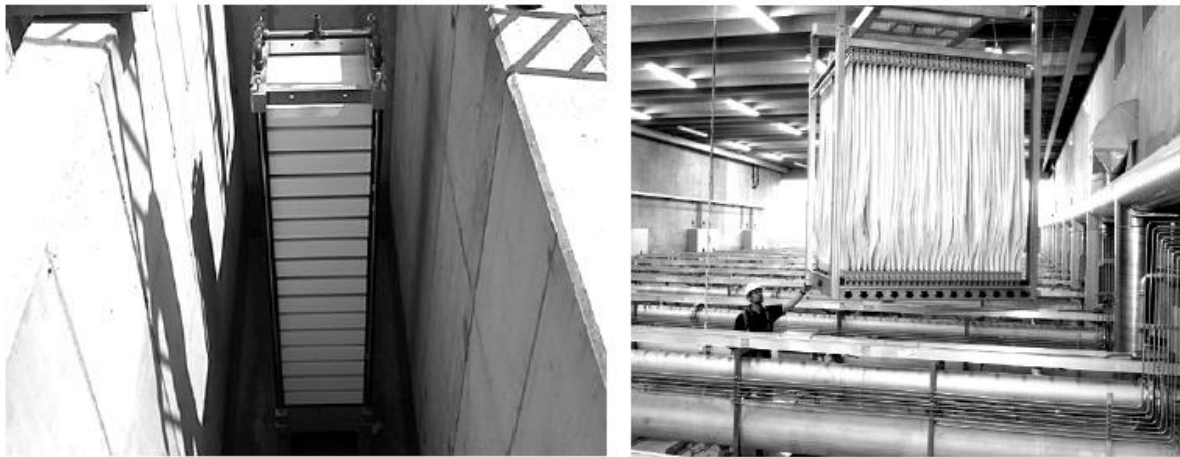
Figure 4-3: Left panel: Ceramic membrane rack inside a membrane basin consisting of 16 membrane modules and a stainless steel frame (Sawatzki 2014); right panel: change of a ZeeWeed 500D polymeric membrane rack consisting of PVDF membranes and a stainless steel frame (GE 2013)
