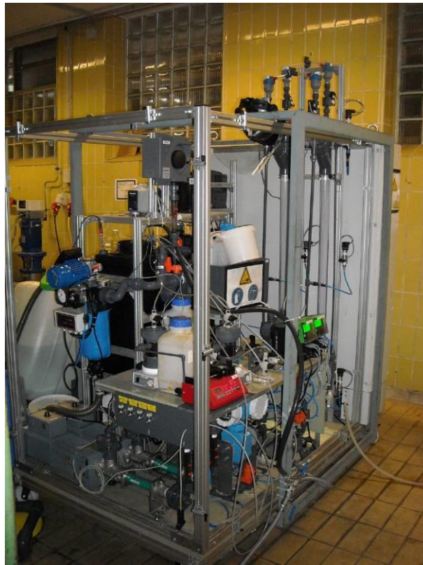
Figure 4-16: UF pilot with two independent treatment lines
